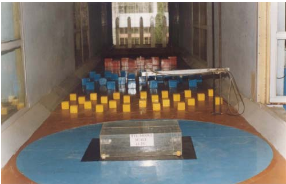
Photo 1 TTU Building Model with Flow simulation Roughness Devices
